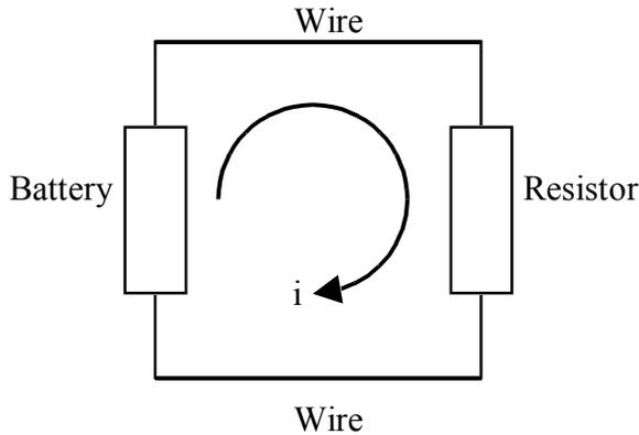
In this elementary circuit, current flows around the circuit in a loop.
