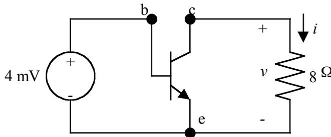
The funny looking symbol is a transistor, a semiconductor device with three points of connection called the emitter, base and collector. We're going to try to amplify a small input voltage, maybe from an antenna, into a signal you can
