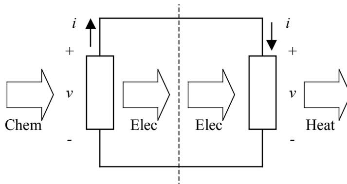
The right element adheres to the passive sign convention. Energy flows in to it from the circuit and is dissipated to the environment. A resistor is the most typical passive element, it converts electric energy to heat energy. The water flow analogy is to head loss in long pipes. The friction of the water appears as heat. (NOT the conductive heat transfer in a heat exchanger!)
