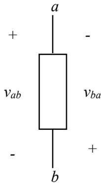
Similarly, voltage is measured between two points, a high point (+) and a low point (-). Knowing which point is the high point and which the low is called *polarity*. (Direction of positive flow is current polarity.) Often the points are given letters or numbers to identify them. These can then be used in subscripts.
