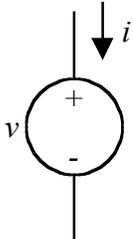
A **voltage source** is a circuit element that controls the voltage across it. The current through a voltage source is determined by the rest of the circuit.
