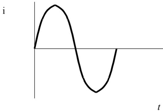
ac current is sinusoidal with respect to time.
