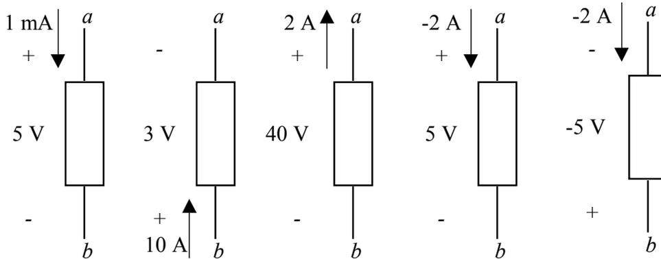
The first one is passive,  $p = 5 \text{ mW}$ , absorbed by element.
