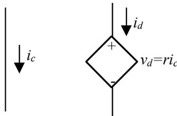
Source voltage  $v_d$  is a linear function of a control current  $i_c$  flowing somewhere else in the circuit.  $r$  is called the gain.
