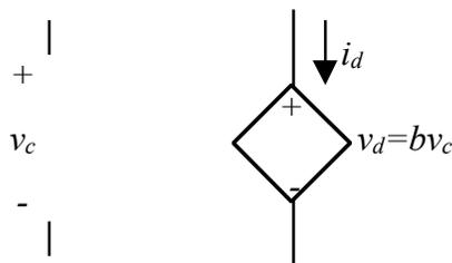
Source voltage  $v_d$  is a linear function of a control voltage  $v_c$  measured somewhere else in the circuit.  $b$  is the gain.
