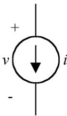
A current source is a circuit element that controls the current flowing through it. The voltage across a current source is determined by the rest of the circuit.
